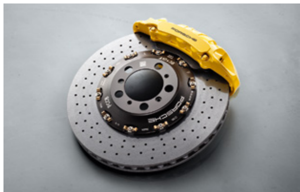
Porsche Ceramic Composite Brake (PCCB)
