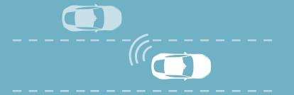
Blind Spot Assist Pack\*\* (Optional<sup>5</sup>) is designed to mitigate the potential for a collision. If another car is in your blind spot when you begin to change lanes, Blind Spot Assist helps to detect the car and applies corrective torque to encourage you to guide your vehicle away from the approaching vehicle. Rear Traffic Monitor uses the same system to alert you, via the Touchscreen, of moving vehicles during reversing.
