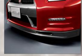
**Evidence of intent.** Designed for the serious business of competition driving, the Track Edition features carbon-fiber ducts on the unique front spoiler to bring additional cooling air to the brakes.
