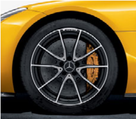
AMG 10-spoke forged wheels with 275/35 R 19 front and 325/30 R 20 rear tyres, painted matt black with a high-shine finish (standard, Code 657)
