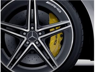
AMG High-Performance Composite Braking System w/ Yellow Brake Calipers (U69)
