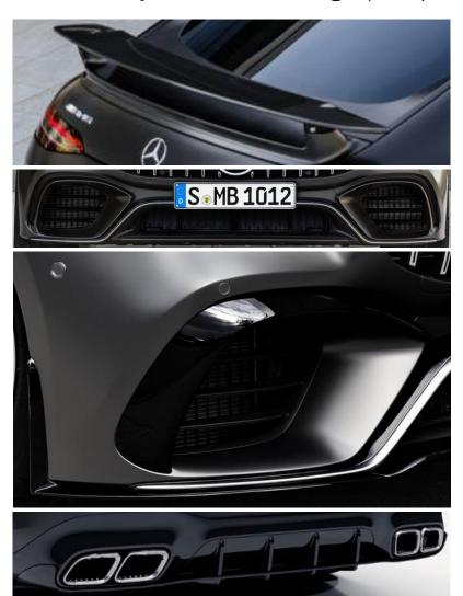
The AMG Aerodynamics package has been developed in the wind tunnel to improve handling at high speeds and provides the basis for even greater driving enjoyment. The attachments increase the negative lift force while reducing drag. The fixed rear spoiler demonstrates a clear commitment to uncompromising performance.
