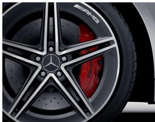
AMG High-Performance Composite Braking System w/ Red Brake Calipers (U70)
