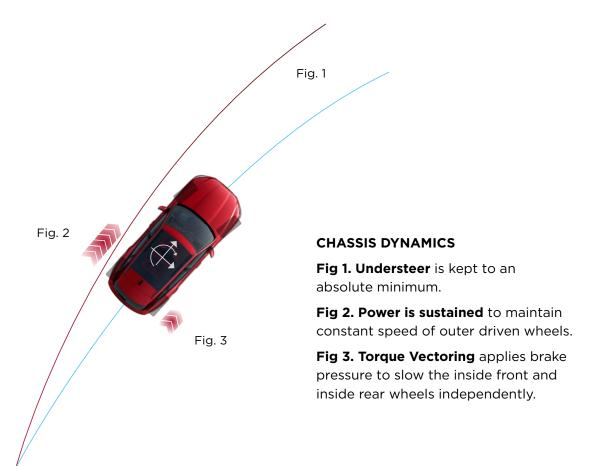
When straight roads become snaking roads, the F-PACE Torque Vectoring by Braking\* makes all the difference. It provides controlled independent braking on the inside front and rear wheels to maximize capability through even the tightest corners. Together with Dynamic Stability Control, it corrects understeer, and provides you with extra confidence when driving.
