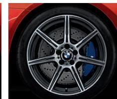
**Double Spoke (Style 601M)** 20 x 9.5 front, 20 x 10.5 rear light alloy wheels and 265/35 front, 295/30 rear **performance tires.**<sup>1</sup>
