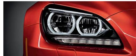
**Adaptive LED Headlights** for both high and low beams project an intense white light that simulates daylight for excellent visibility. Convenient features that improve visibility include Automatic headlights, Adaptive turning, Cornering Lights, four Corona headlight-rings, and Automatic high beams.
