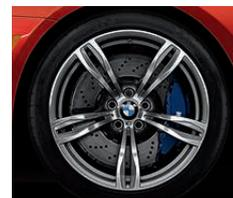
**Double Spoke (Style 343M)** 20 x 9.0 front, 20 x 10.0 rear forged light alloy wheels and 265/35 front, 295/30 rear **performance tires.**<sup>1</sup>
