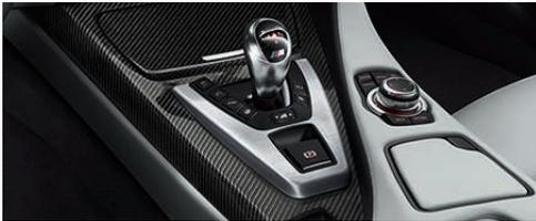
**Gear shift lever** for 7-speed M Double Clutch Transmission with Drivelogic includes M logo and illumination.
