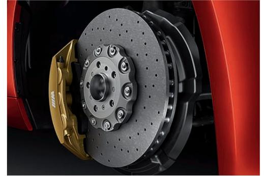
**M Carbon Ceramic Brakes** in the BMW M6 Coupe and Convertible have an extremely high load capacity and excellent resistance to fade. The system can be identified by the gold brake calipers with M logo.
