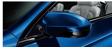
**M side-view mirrors** in body color are heated and electrically adjustable. The mirror base and lower part of the mirror case are painted in high-gloss black.
