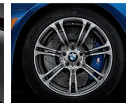
**Star Spoke (Style 344M)** 19 x 9.5 front, 19 x 10.5 rear forged light alloy wheels and 265/40 front, 295/35 rear **performance tires.**<sup>1</sup>
