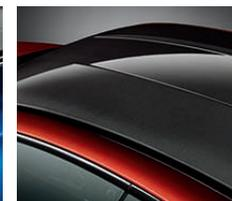
**Carbon fiber roof** of the M6 Coupe is made of carbon fiber reinforced plastic (CFRP). Very light and extremely stiff, it lowers the vehicle's center of gravity for enhanced handling, especially when cornering.
