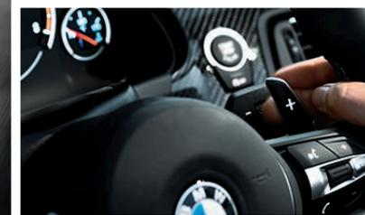
Racecar technology: the 7-speed M Double Clutch Transmission with Drivelogic can be shifted in a flash, using paddles. Just as in advanced racecars, you can keep your foot firmly on the throttle while shifting. Whether shifting up or down, engine revs are perfectly and instantly matched to the next gear.
